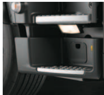
Manoeuvring light in co-driver's entry lights up the visible area of the ramp mirror.
