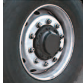
MAN HydroDrive® wheel hub motor.
