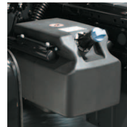
Separate AdBlue® tank for construction vehicles.
