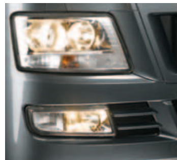
Headlights with free-form reflectors, Xenon dipped headlight.
